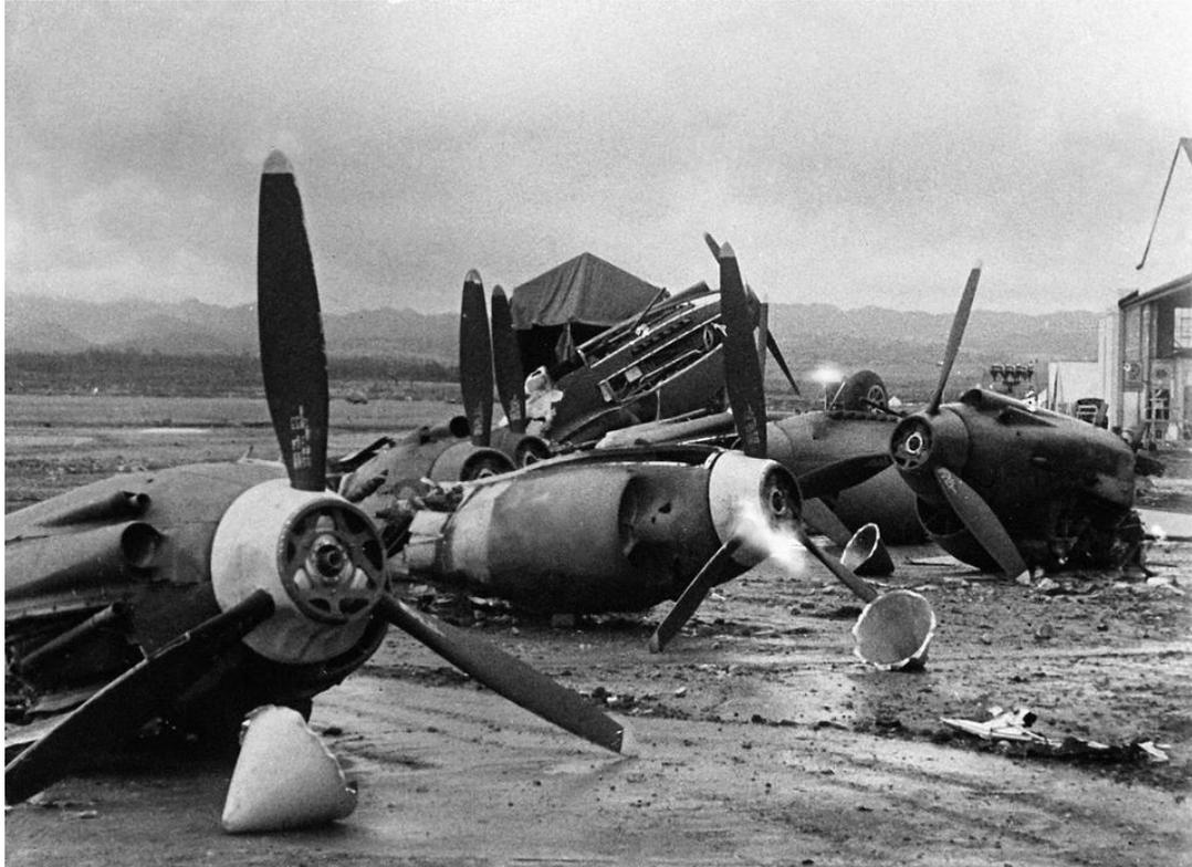
***A Sad sight, P-40B/Cs, destroyed at Wheeler Field being salvaged: note spinners are off.***
