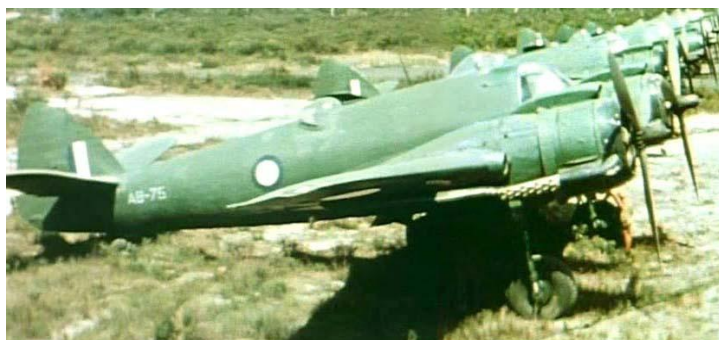
Foliage Green Beaufighter 21s (A8-75 left), with black collector rings 154
