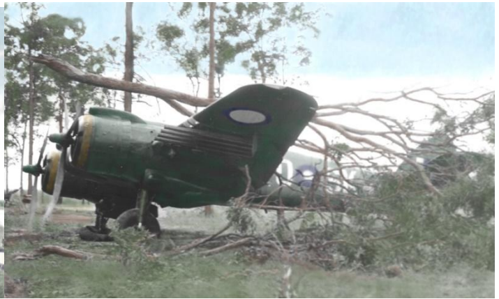
A8-119 SK-O, 19 APR 45 tyre blew on landing at
