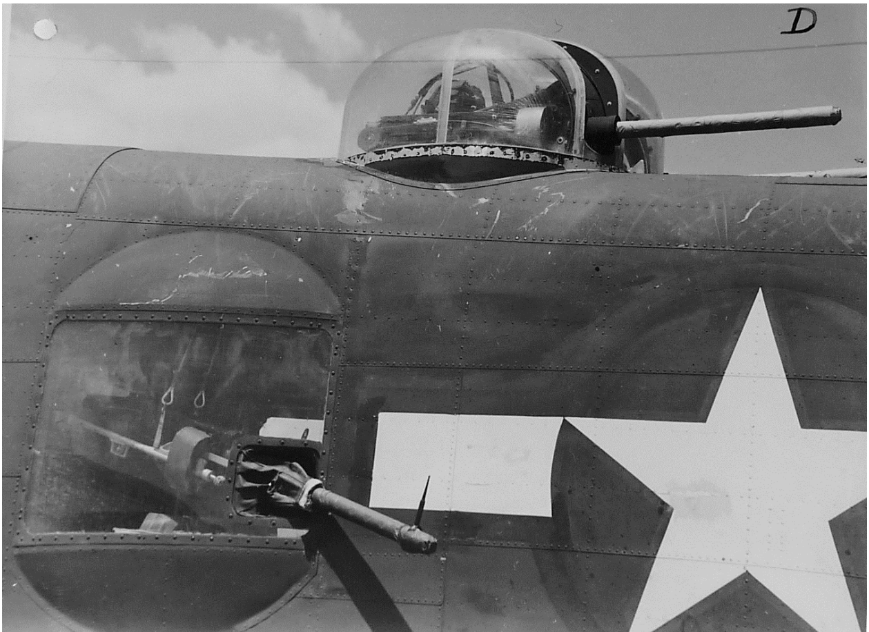
This is the port-side waist gunner's position. The starboard side position was identical and occupied the same fuselage stations. These were factory installed on the production line and NOT a modification centre installed accessory, the only changes made by the modification centre by this stage in B-25D production was the actual installation of the weapons and some internal fittings. [NAA: A11093, 452/A47].
