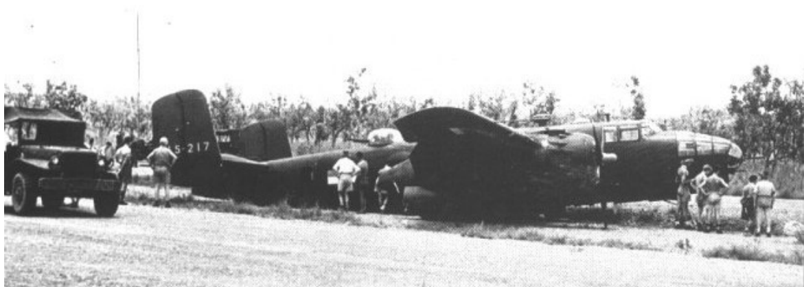
This is N5-217 (serial clearly visible on vertical stabilizer) after a mishap at Pell on 09FEB45. This picture has been quoted as being of B-25J, 43-27925, which is obviously incorrect. All of the NAA model NA-100 diagnostic features are visible to prove that this simply cannot be a model NA-108 (B-25J): Consolidated twin-50 package guns, astrodome at navigator's station (immediately behind cockpit), large fairing above starboard side waist gunners window, dorsal turret aft of trailing edge of wing and steeper fairing for tail gunner's position. This aircraft is a B-25D and most likely a B-25D-35-NC. I believe it is either the former 43-3620 or 43-3765. [Image via ozatwar.com/ozcrashes/nt130a].
