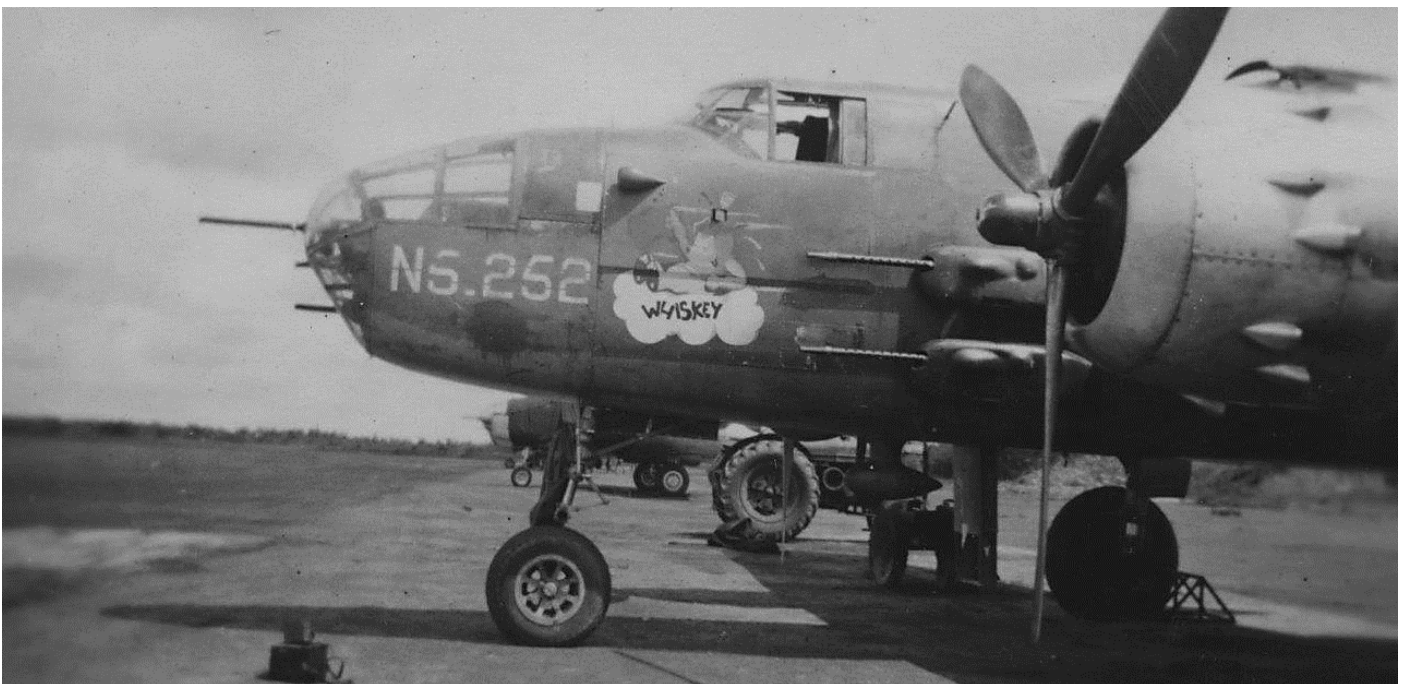
This is 18(NEI)SQN's N5-252 at an unidentified location in (I believe) 1946. It is wearing OD uppers. The port engine cowling has been stripped of paint and, although it is difficult to tell with certainty, the undersides seem to have been similarly treated. The bare metal on the engine cowling is dull from exposure. The next aircraft in line is a B-25 in natural metal finish. N5-252, a B-25J-25-NC, was received by 18(NEI)SQN on 12MAY45, too late to participate in any operations from Australia. Another interesting point visible in this image is the blisters on the package guns. This type having two blisters, the larger, forward, blister fairing over the link ejection chute and the smaller blister just aft of it fairing over the guns firing solenoid. [Collection Netherlands Institute of Military History item 2002-336-41 via nimh-beeldbank.defensie.nl ].
