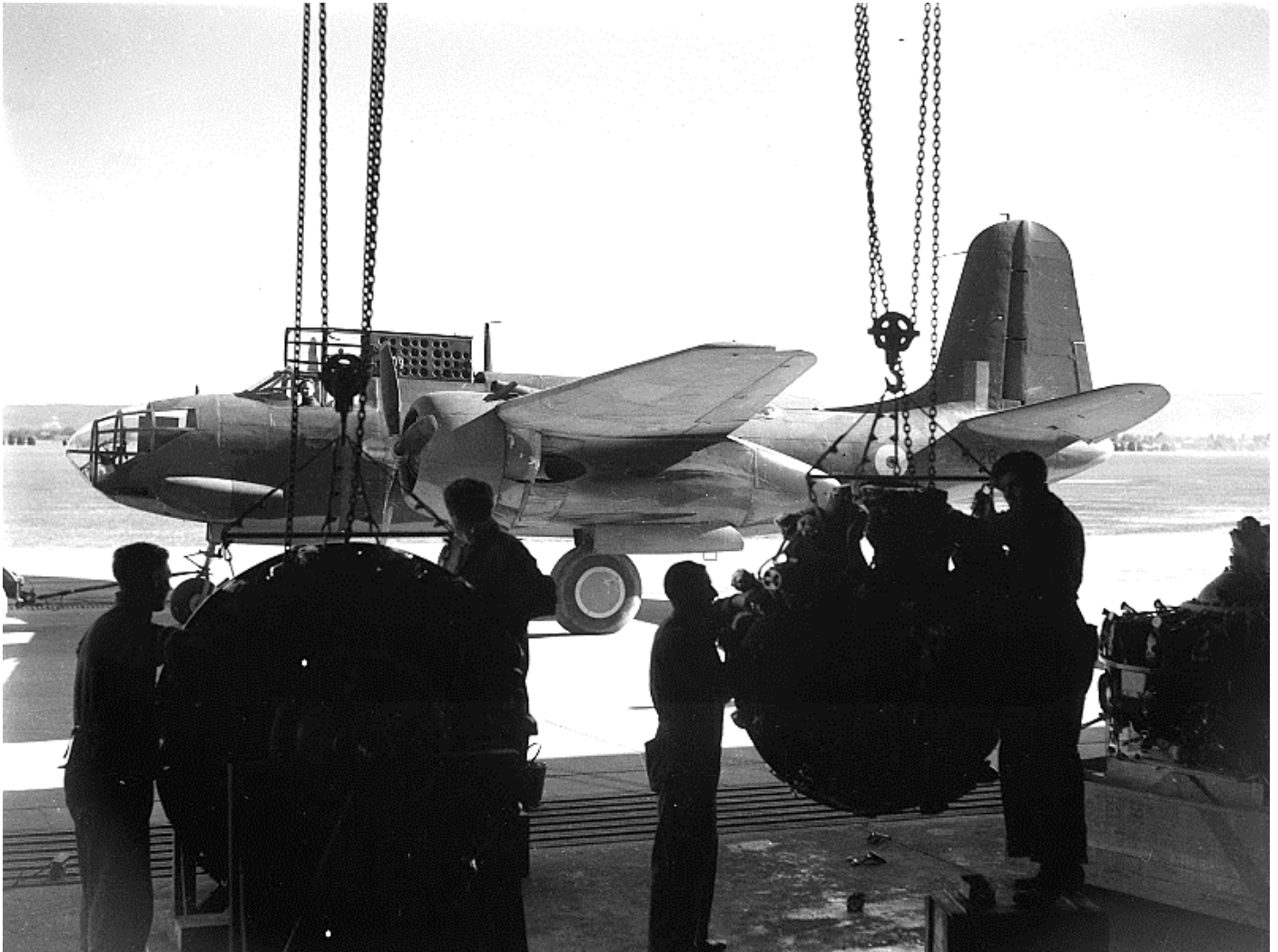
Newly assembled DB-7B Boston III at 2AD Richmond, new Wright Cyclone Engines removed for modification to be refitted to Bostons. [Daniel Cox collection].
