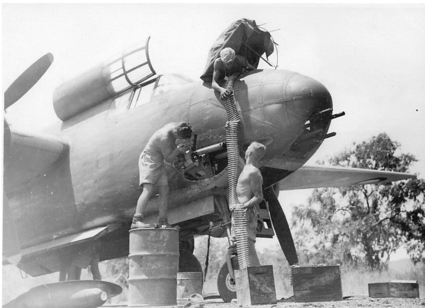
DB-7B Boston after modification to a straffer, 4 x .50 MGs thru nose and 4 x .303 MG cheek guns. [22 Squadron Association].
