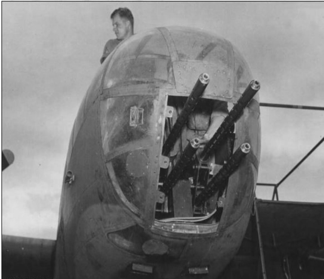
The same mounts and installation were used in A-20A/DB-7B and B-25C/D for Pappy Gunn's 4 x .50 installation. This is a B-25C/D .50 installation. [22 Squadron Association].
