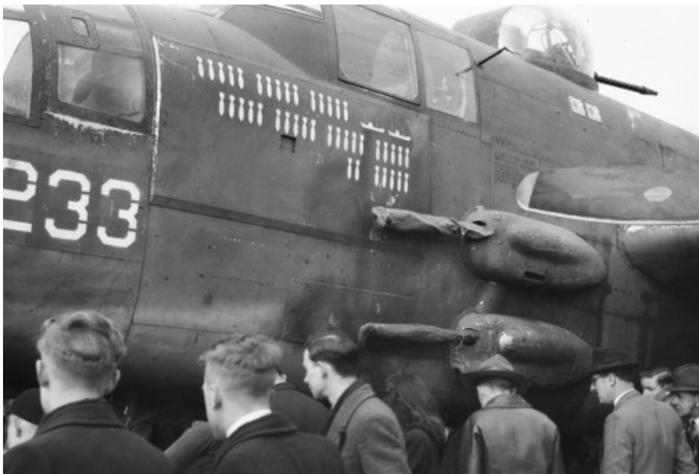
This is N5-233/GM-W, a B-25J-15-NC, photographed during a display in Victoria and shows the two individual package guns fitted to NA-108 aircraft. Notice the large blister type fairing of this later style which made room for the link chutes. Also, the angled fairing between the two gun packs which covered the chute for the link from the top gun to the common link ejection opening on the underside of the lower pack. Compare the single, large, blister of these package guns with those that appear on N5-252 back on p78. [AWM image 114122].
