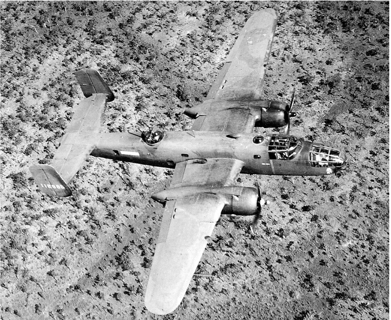
This is 18(NEI)SQN's N5-134, ex 41-12885, a B-25C. It seems that a disruptive scheme had been applied across the upper surface of the wing and across the fuselage centre section as well as the vertical stabilisers. It is difficult to tell if a pattern had been applied to the horizontal stabilizer, although some mottling seems to have been applied to the leading edge on the starboard side. The wedge shape discolouration immediately below the dorsal turret is likely caused by the use of a protective tarpaulin over the turret. [Aviation Heritage Museum of WA image P021898 via Mike Mirkovic].
